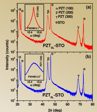
XRD patterns of PZT films on STO substrates grown by (a) dual and (b) single-laser ablation, respectively. Insets show the rocking curves about the PZT (100) peak.
