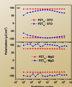
Fatigue tests at 10 kHz using  $\pm 9 \text{ V}$  read/write voltages for LSMO/PZT/LSMO capacitors.
