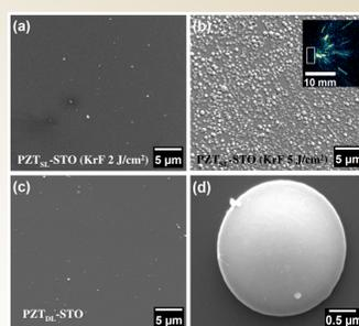
SEM images of single laser PZT films on STO substrates ( $\text{PZT}_{\text{SL}}$ ) at (a) low fluence of  $2 \text{ J/cm}^2$  and (b) high fluence of  $5 \text{ J/cm}^2$ , and (c) dual laser film ( $\text{PZT}_{\text{DL}}$ ), (d) one of the "splashed" particulates on  $\text{PZT}_{\text{SL}}$  film ejected from target.
