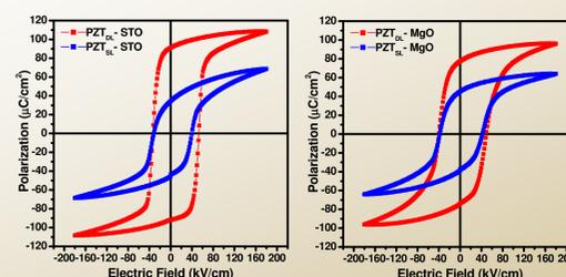
P-E hysteresis loops for PZT films deposited using DLD ( $\text{PZT}_{\text{DL}}$ ) and single laser ablation ( $\text{PZT}_{\text{SL}}$ ) on STO and MgO substrates.
