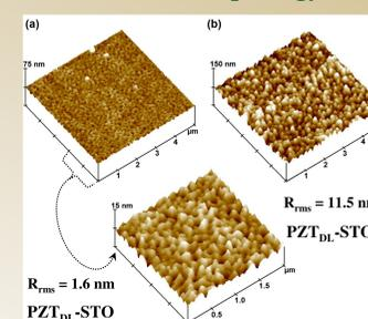
AFM images of PZT films on STO substrates deposited using (a) dual-laser ( $\text{PZT}_{\text{DL}}$ -STO), and (b) single-laser ( $\text{PZT}_{\text{SL}}$ -STO) ablation, respectively.
