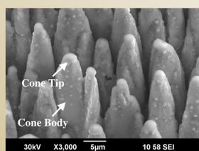
SEM image of conical structures formed on a PZT target surface after repeated ablation by KrF excimer laser.
