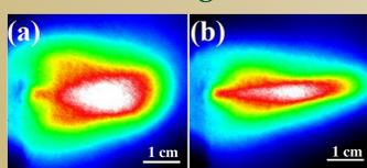
Time integrated ICCD images of the visible emission spectra of laser-induced plumes in 500 mT ambient  $\text{O}_2$  for (a) dual-laser ablation, and (b) the KrF single-laser ablation.
