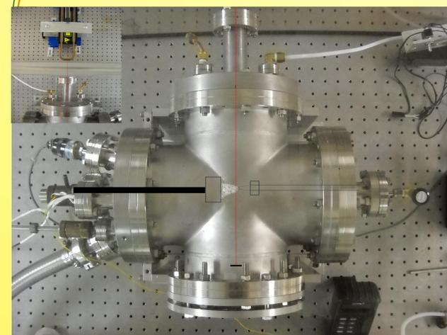
Laser Assisted Spray process top-view with diagram depicting the internal action of the process. The beam entering from the top of the picture, intercepts the aerosol in order to remove the surfactant coating of the PbSe.
