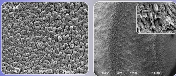
Scanning electron microscope images of (left) non-ablated central region of the target and an (right) ablated track with an inset at 1000x to illustrate the conical formations at the target surface after several hundred thousand pulses.
