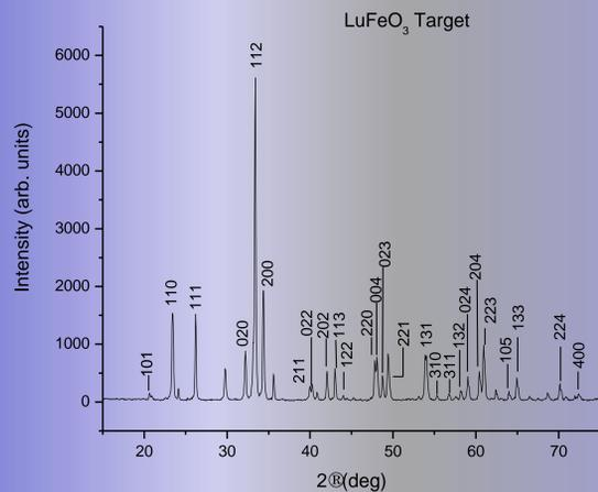
XRD analysis shows the  $\text{LuFeO}_3$  phase for the stoichiometric target.
