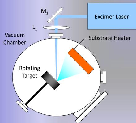
Schematic of the pulsed laser deposition chamber depicting the Excimer laser source with the focusing optics and rotating target holder. A heated substrate facilitates the mobility of the arriving species and nucleation of critical binding sites.
