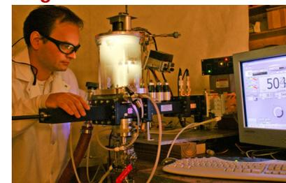
Microwave plasma deposition of nanoparticle coatings
